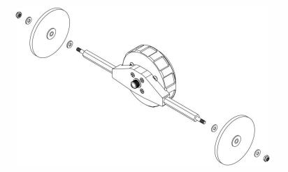
Remove outer wheels using 7/16" wrench
