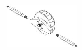
Remove axles using 1/2" wrench
