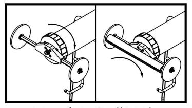
Screw on front cap assembly & nozzle
